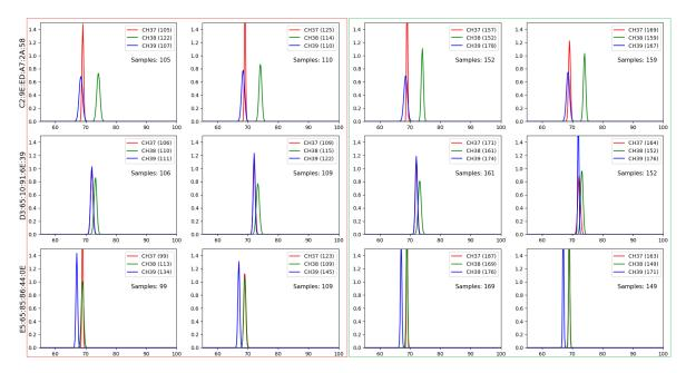
Figure 2.17: Impact of multiple beacon transmissions to the detection response. (Total transmitting beacons at Left Group: 60 beacons vs Right Group: 3)
