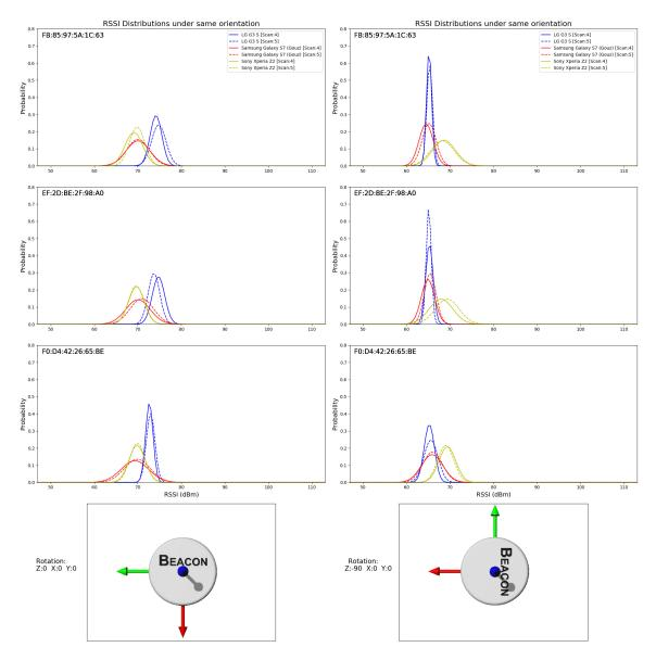
Figure 2.12: Comparing the signal of three different Beacons, while having 2 different orientations
