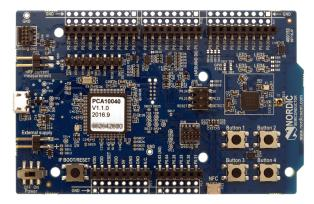
Figure 2.14: nRF52 Development Kit from NORDIC SEMICONDUCTOR
