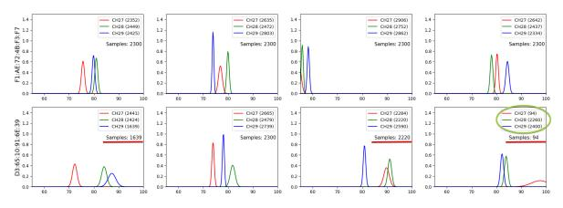
Figure 2.15: LG G3 RSSI records at channel level, from 2 (out of 20) different beacons. The 4 plot columns correspond to the 4 different positions used.
