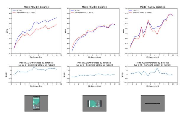
Figure 2.13: Comparing the RSSI difference (based on distance), between 2 phones
